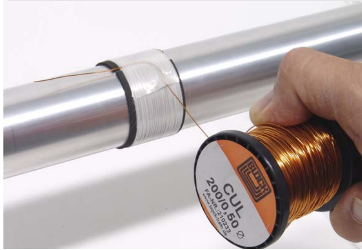
Coil, depends of shaft diameter 8-13 paralle windings of 0.5 CUL wire
