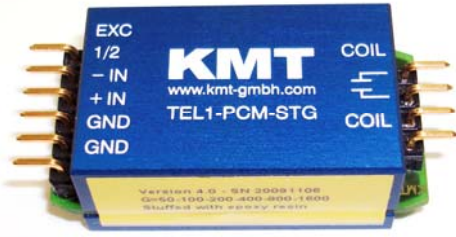
New version 4.0 without external CAL pins
