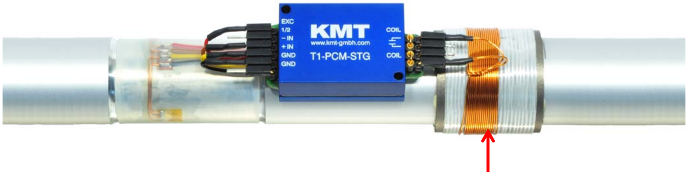
Coil, depends of shaft diameter 5-18 windings of 0.5 CU wire
