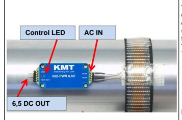
The pins "AC IN" are the AC power input from the coil. On the pins "+6.5" and "GND" you get a stabilized output voltage of 6.5V DC. The control LED will lights up, as soon as the power head is switched on and at the right position - close enough to the coil on the shaft. The max. load current on the DC output is 100mA. The AC/DC converter will use instead battery pack!
