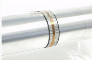
Wind the 0.5 mm enameled copper wire around the shaft:
