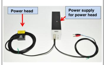
Connect the power head on the "AC Out" socket of the power box and then the DC power cable on the "DC In 10-30V" socket. The two banana plugs have to be connected to a DC power source with red on +10-30V DC and **black** on **0V**.
