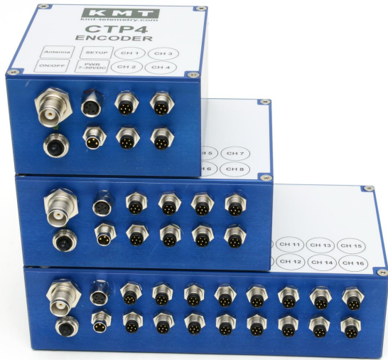
4,8 and 16-CH encoder in IP65 Aluminum housing
