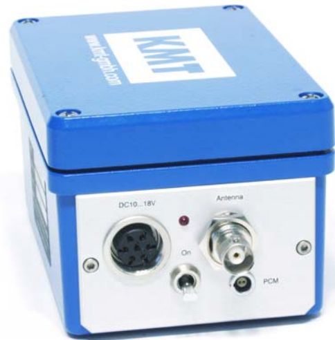
Back side with power In and antenna Out
