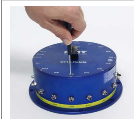
Untwist to open the housing with hexagon screw driver 2mm
