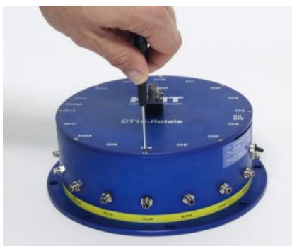
Untwist to open the housing with hexagon screw driver 2mm
