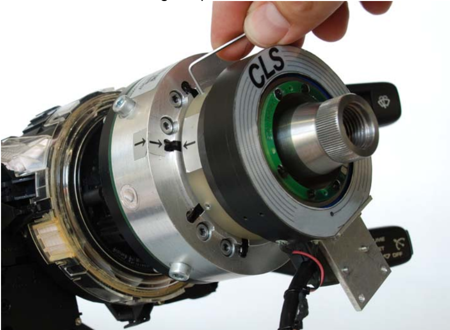
Assembly of the encoder
