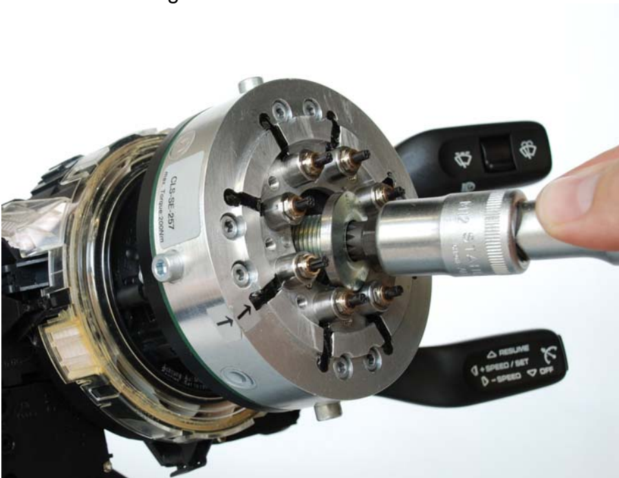
Assembly of the sensor
