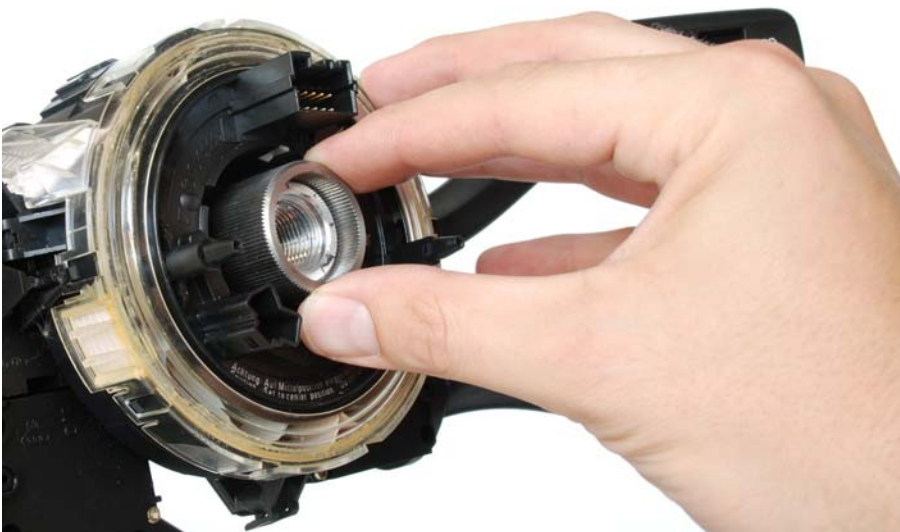
Assembly of the steering column adapter
