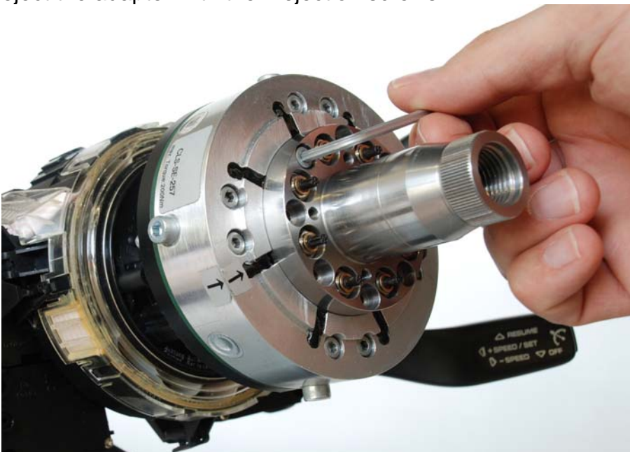
Assembly of the steering wheel adapter
