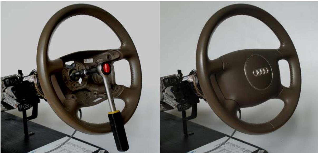
Assembly of the steering wheel
